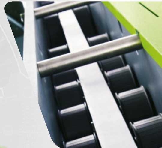
Roller drive with 2 servomotors
