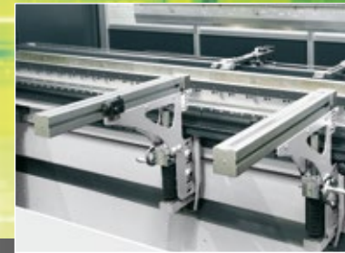
Moveable support arms adjustable in height
